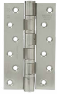
BHP 2765SS 6"X3,5"X4MM 5BB NRP 100KG/PAIR
