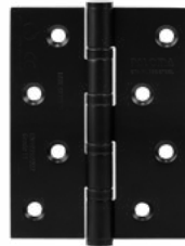
BHP 3741MB 4"x3"x2MM 4BB NRP 50KG/PAIR
