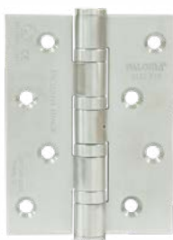
BHP 112 4"X3"X4MM 4BB NRP (NEW) 90KG/PAIR
