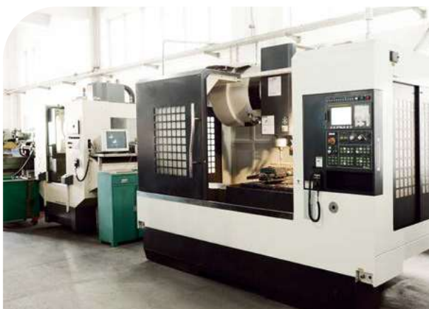
Automatic CNC machining centers to ensure high precision of inner structure.
