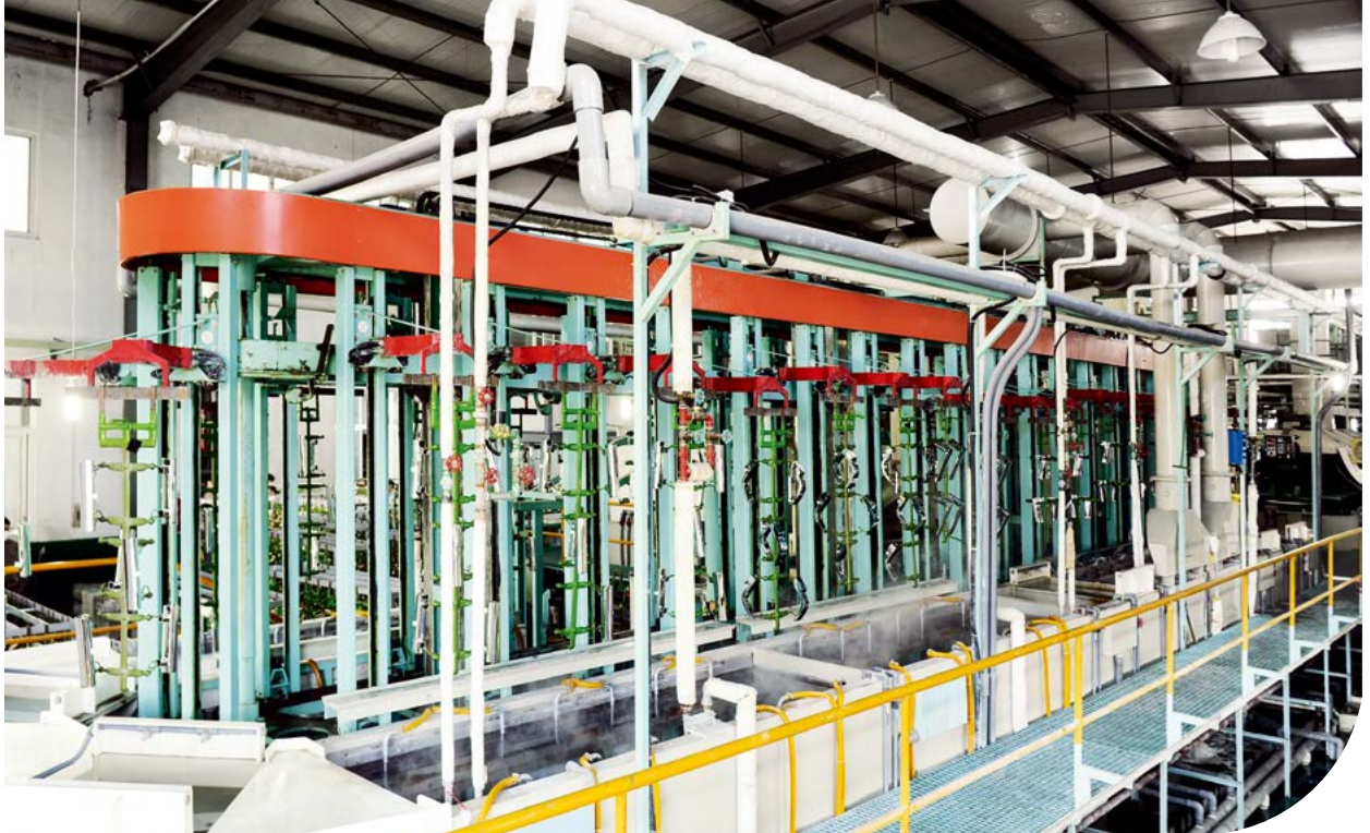
Automatic plating lines to ensure the stability of the highest quality product finishes that can never be achieved using manual methods.
