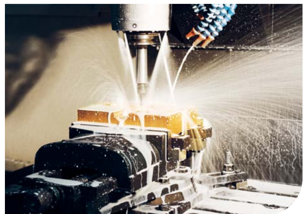
80% of the machining procedure done at one setting due to efficient computerized programming and large capacity of the tool magazine.
