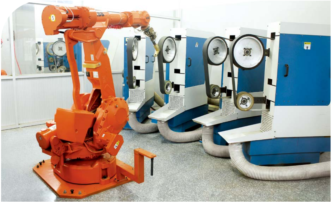
Automatic robotic polishing to guarantee a perfect finish on every product.
